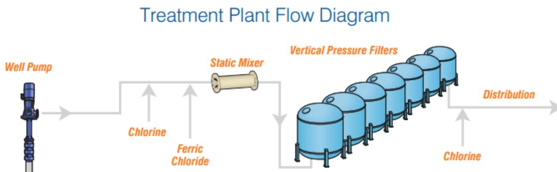
**Figure 1. Water Treatment Configuration for Arsenic Removal (WesTech)**
