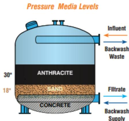
**Figure 2. WesTech Pressure Filters for Arsenic Removal**
